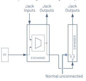
With this configuration, the jack outputs of Exchange are duplicated to the jack outputs of Expander. The jack outputs and chain outputs of Exchange are independently buffered, so the loading on one output bank by connected modules will not affect the other.
