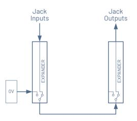
The figure below shows how the normal connections can be used to chain multiple Expanders together. The normal connected Expanders provide multiple points in the chain which can be broken by inserting a jack. The rightmost jack in the input Expanders in the chain will drive the outputs of the output Expander.
