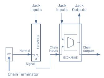
inputs or the corresponding jack inputs on Expander, and feed the selection into its switching matrix.
