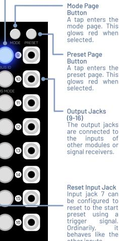
Input jack 7 can be configured to reset to the start preset using a signal. it behaves like the other inputs.
