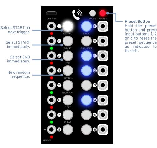
The sequence reset functions will have no effect in the preset input CV mode. The behaviour is the same for random sequences, except the random sequence will continue with a random preset on the next trigger after the reset function has completed. While PRESET is held down, buttons can be pressed multiple times to reset a sequence during a live performance.
