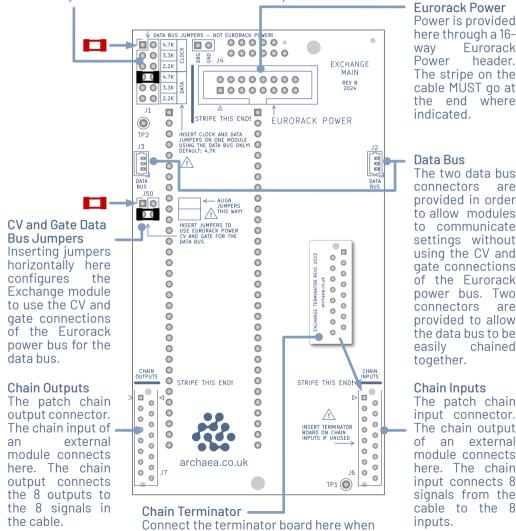
the chain inputs are not connected.
